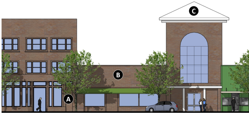
Figure 3-2: Building Base, Middle, and Cap
