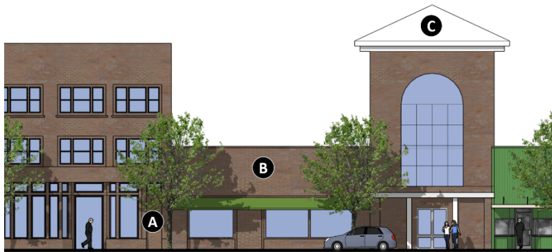
Figure 3-2: Building Base, Middle, and Cap
